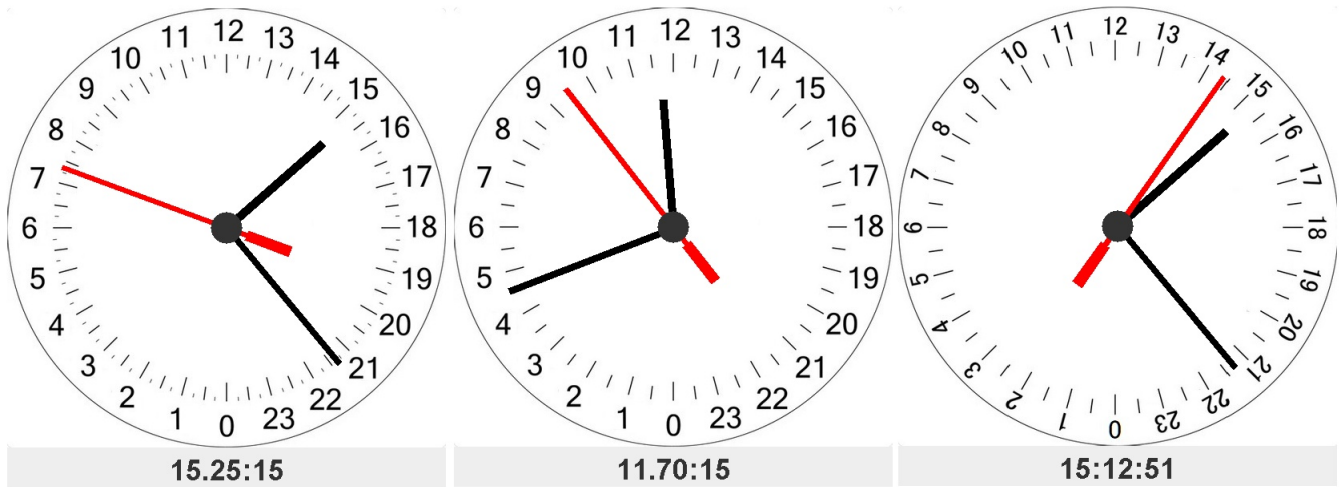
Figure 2. Three desktop clockfaces. Left: the “exact” Martian clock, the second hand sweeps once per each “minute” (hundredth-of-an-hour); Middle: the “relaxed” Martian clock, the second hand sweeps once per two “minutes”; Right: the Space Clock, for free-floating crew.
